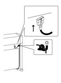
**10.** Insert the pedal connection cord that comes from Pedal Board into the main unit's pedal jack and fix with the clamp of the Side Panel.
